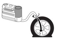
Note: When the sealing compound is first added into the tire, the air pressure gauge reading on the compressor unit may indicate a higher value; this is normal and should be no reason for concern. The pressure will drop after about 30 seconds of operation. The
